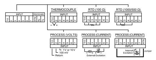
**Figure 2.3 Rear Panel Input Connections**
